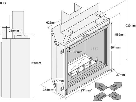
\* Includes the required 25mm clearance to each side and rear of the fireplace
